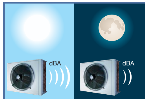
Time-based condenser fan noise reduction
